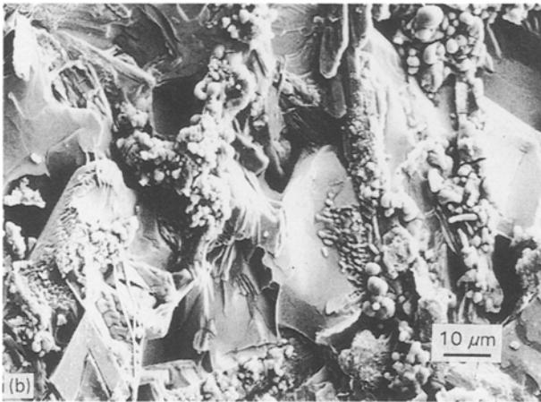
Figure 3 Microstructure of (a) sintered BPSCCO strips, and (b) strips heat-treated at 860 °C.
